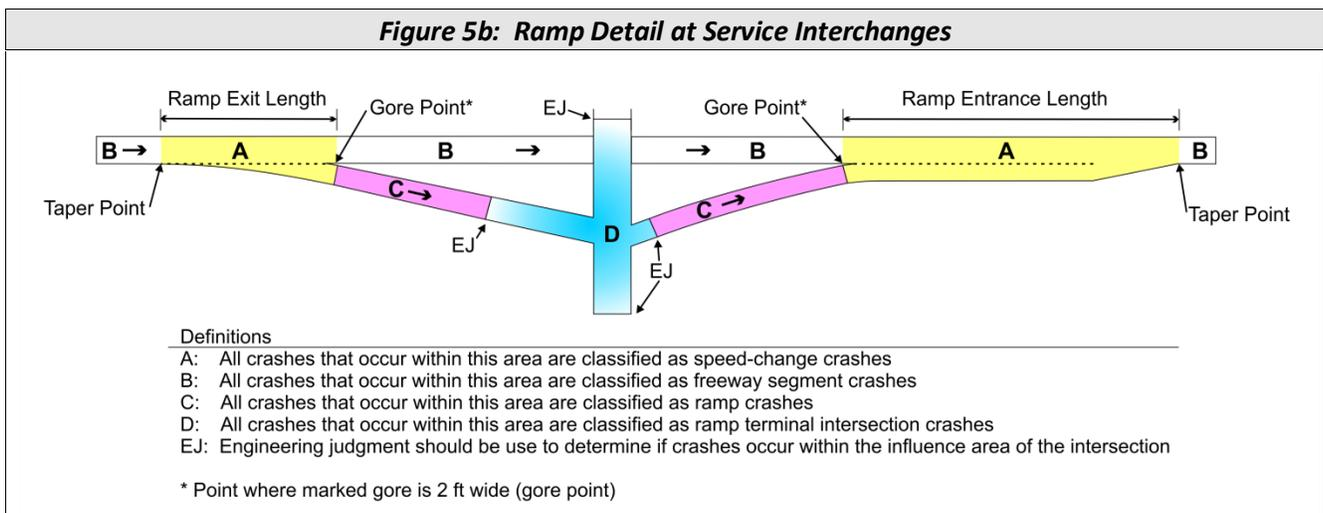
The definitions shown in **Figure 5b** for speed-change areas and freeway segments are based on definitions in the Enhanced Interchange Safety Analysis Tool (ISETe): User Manual, published May 31<sup>st</sup>, 2012 through the National Cooperative Highway Research Program (NCHRP). **Figure 5b** also includes guidance about defining ramps and the influence area of intersections, which are definitions specific to WisDOT business practices.
