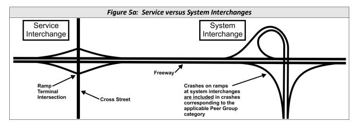
At service interchanges, the variability in ramp designs and interchange configurations present challenges for conducting consistent analysis. If crash analysis is conducted at a service interchange, it is suggested the analysis be conducted using the segmentation shown in *Figure 5b*.
