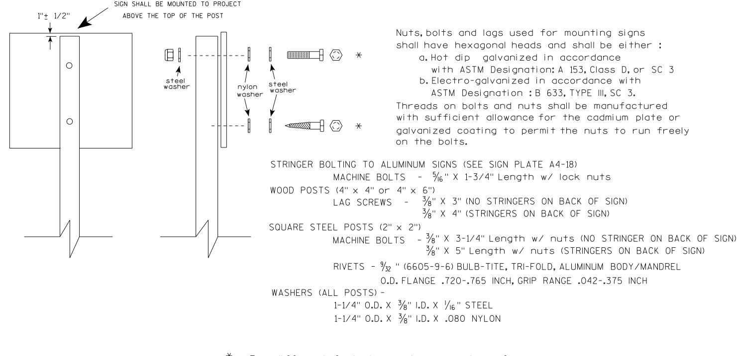
Two different fastening systems are shown for illustration purposes. On any individual sign, either one or the other system shall be used. Actual number of fasteners per sign varies with the sign area, but normally there are two. For a single post installation, all signs greater than 9 sq.ft. require the use of 3 fasteners.
