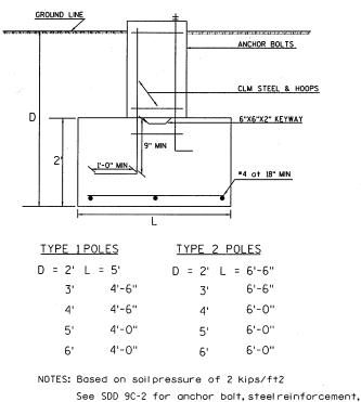
See SDD 9C-2 for anchor bolt, steel reinforcement conduit and other requried details.
