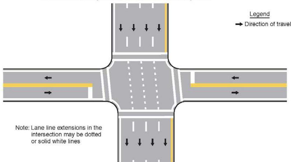
**B - Typical pavement markings with double-turn lanes, lane-use turn arrows, and optional crosswalk lines, stop lines, and line extensions into intersection for double turns**
