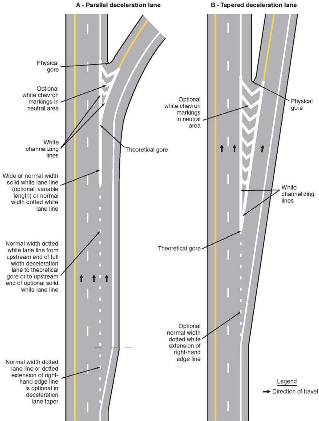
**Figure 3B-8. Examples of Dotted Line and Channelizing Line Applications for Exit Ramp Markings (Sheet 2 of 2)**
