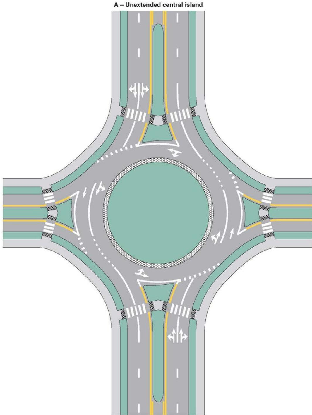
**Figure 3C-4. Example of Markings for a Two-Lane Roundabout with One- and Two-Lane Approaches (Sheet 2 of 2)**
