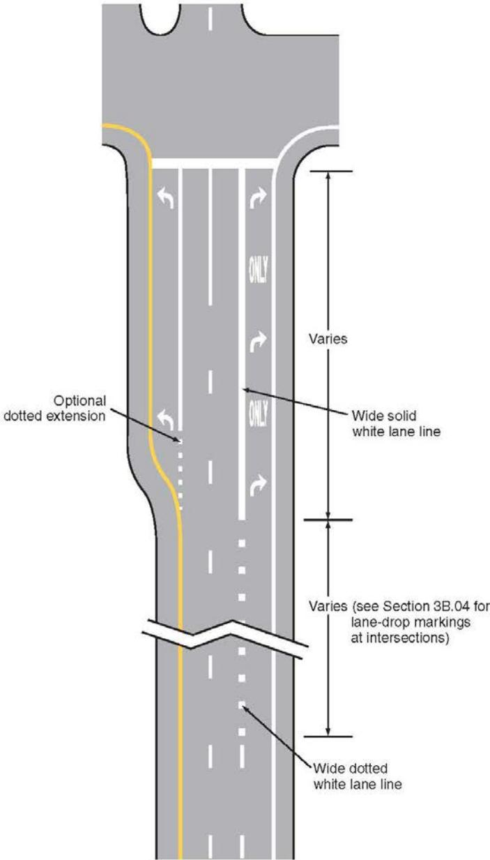
**Figure 3B-11. Examples of Applications of Conventional Road Lane-Drop Markings**
