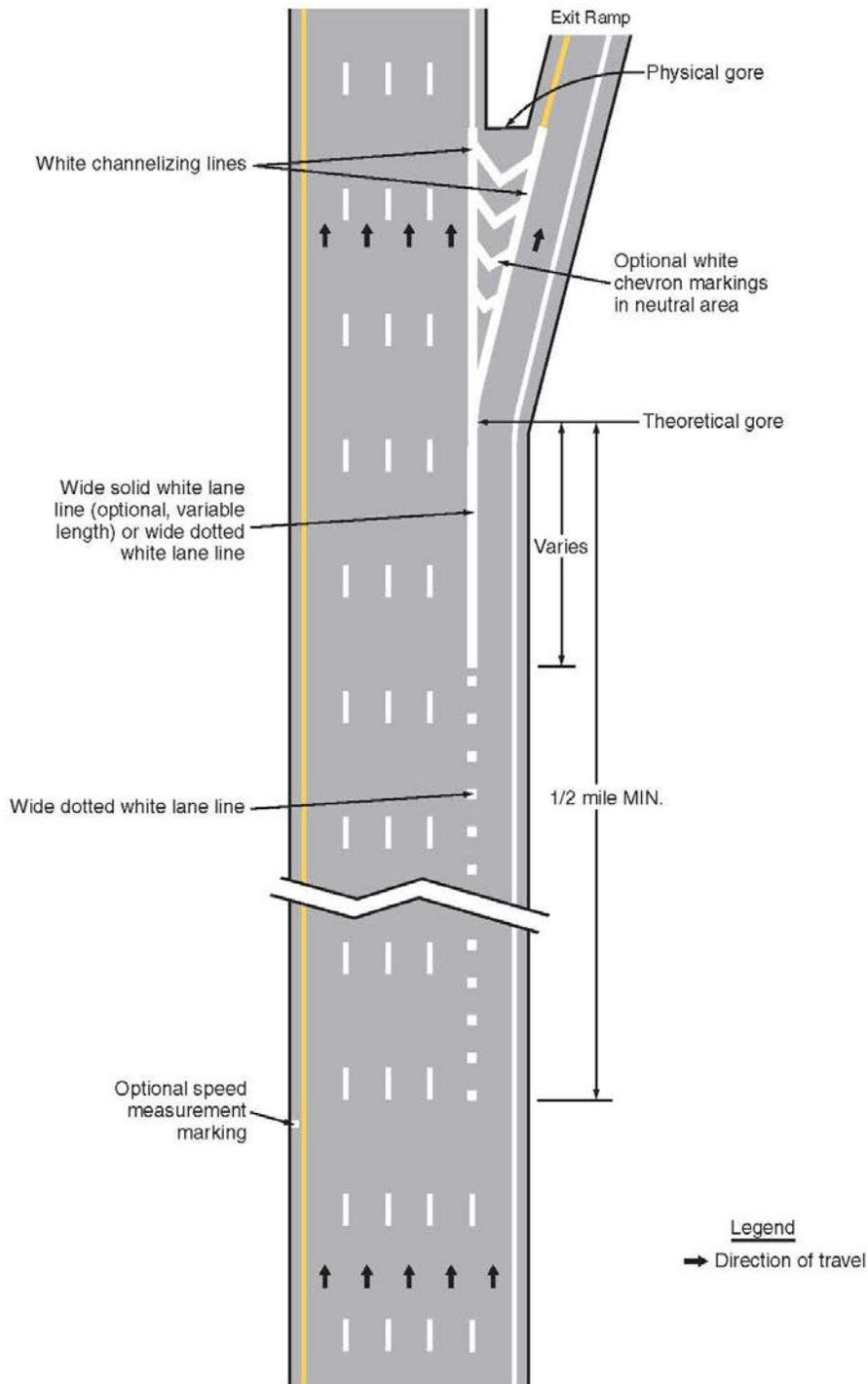
**Figure 3B-10. Examples of Applications of Freeway and Expressway Lane-Drop Markings (Sheet 2 of 5)**
