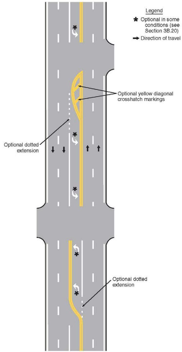
**Figure 3B-3. Examples of Three-Lane, Two-Way Marking Applications**
