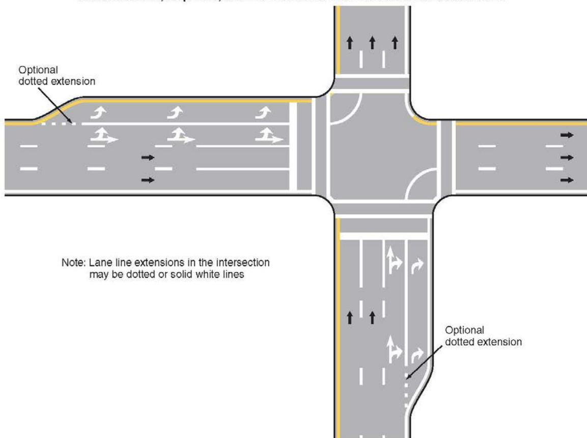
**Figure 3B-13. Examples of Line Extensions through Intersections (Sheet 2 of 2)**
