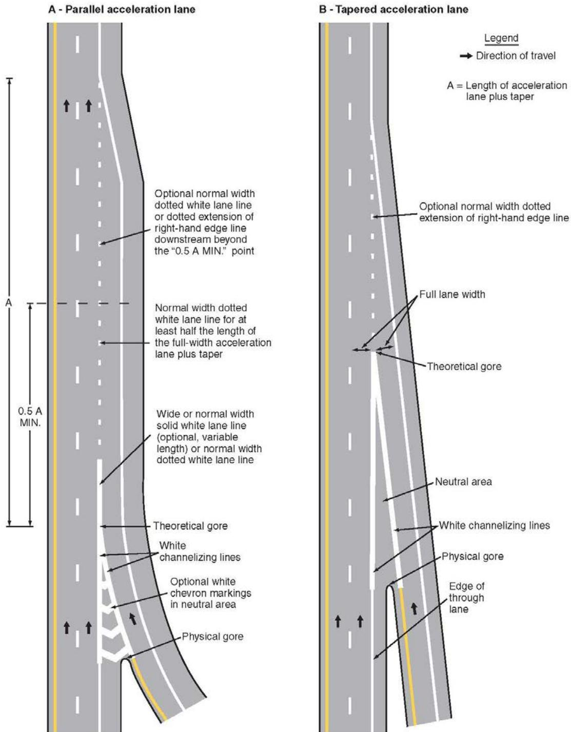
**Figure 3B-9. Examples of Dotted Line and Channelizing Line Applications for Entrance Ramp Markings (Sheet 2 of 2)**
