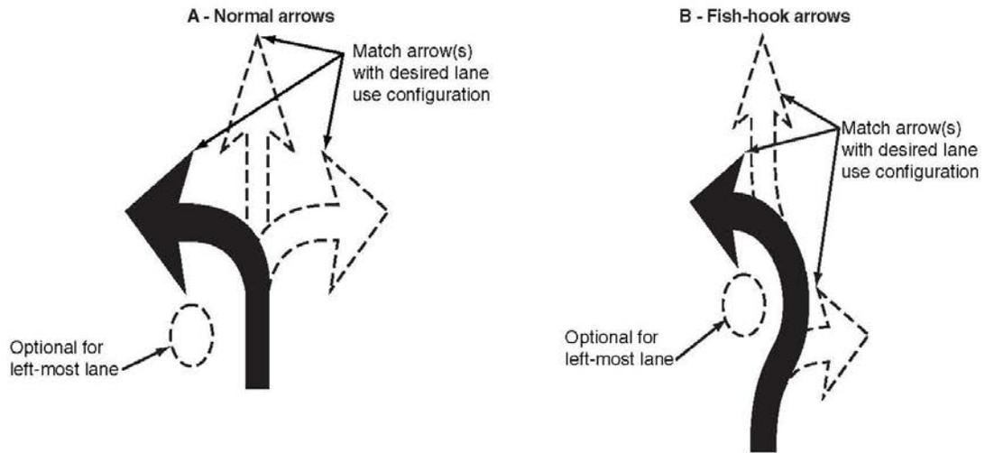
**Figure 3C-3. Example of Markings for a One-Lane Roundabout**
