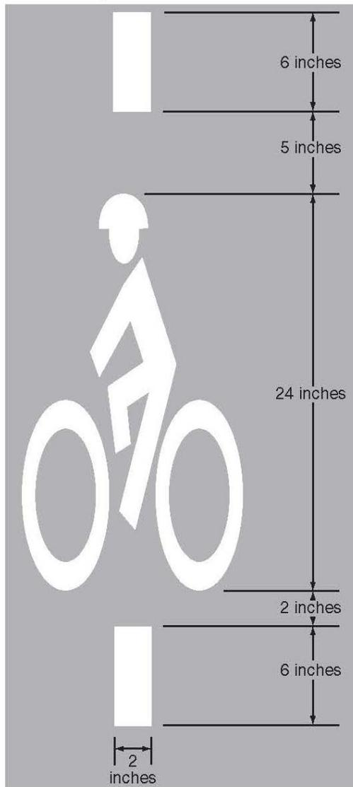
**Figure 9C-8. Examples of Obstruction Pavement Markings**
