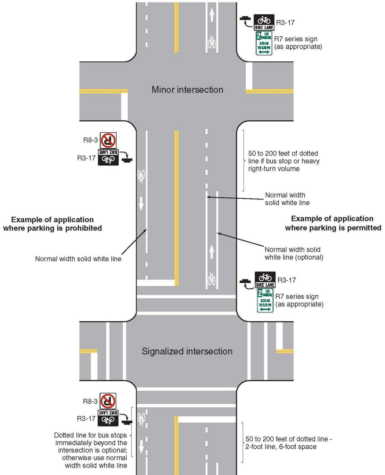
**Figure 9C-7. Bicycle Detector Pavement Marking**
