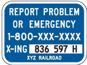
Figure 8B-5. Example of an Emergency Notification System Sign
