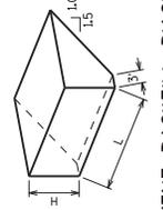
**ABUTMENT BACKFILL DIAGRAM FOR WINGS PARALLEL TO ROADWAY**
