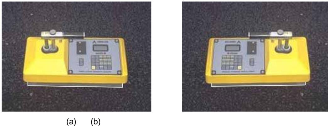
**Figure 2: Nuclear gauge orientation for (a) 1<sup>st</sup> one-minute reading and (b) 2<sup>nd</sup> one-minute reading**
