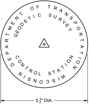
GEODETIC SURVEY DISC FURNISHED BY WISDOT
