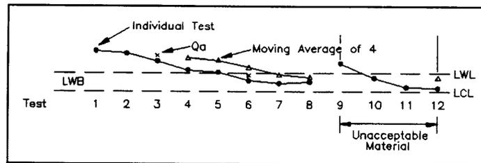
**EXAMPLE B:** The Contractor notified the Engineer at test 7. At test 8, the Contractor and Engineer discuss an action to take. At test 12 the new moving average is still within the warning band and the material represented is unacceptable and will require correction before subsequent fill placement.
