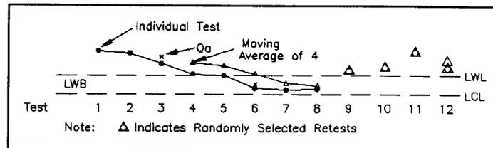
**EXAMPLE C:** The Contractor performs additional corrective actions on the unacceptable material (test 9-12). A re-test of the corrected material is used in calculating the new moving average for point 12. The new moving average is now above the warning limit and the Contractor continues fill placement.
