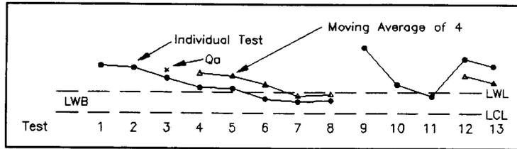
**EXAMPLE A:** The Contractor notifies the Engineer at test 7. At test 8 the Contractor and Engineer discuss an action to take. At test 9 the new moving average of 4 random tests begins. At test 12 a new moving average is established, if this moving average is above the warning limit and the Contractor continues fill placement with the problem, seemingly, resolved.
