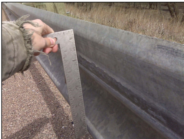
FIGURE 625-9 Rail Damage Examples Flattened Rail
