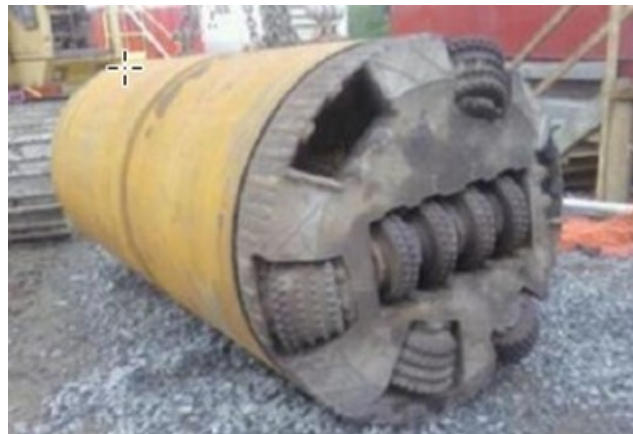
Figure 20.2 Microtunneling Machine (Source AASHTO TC3)
