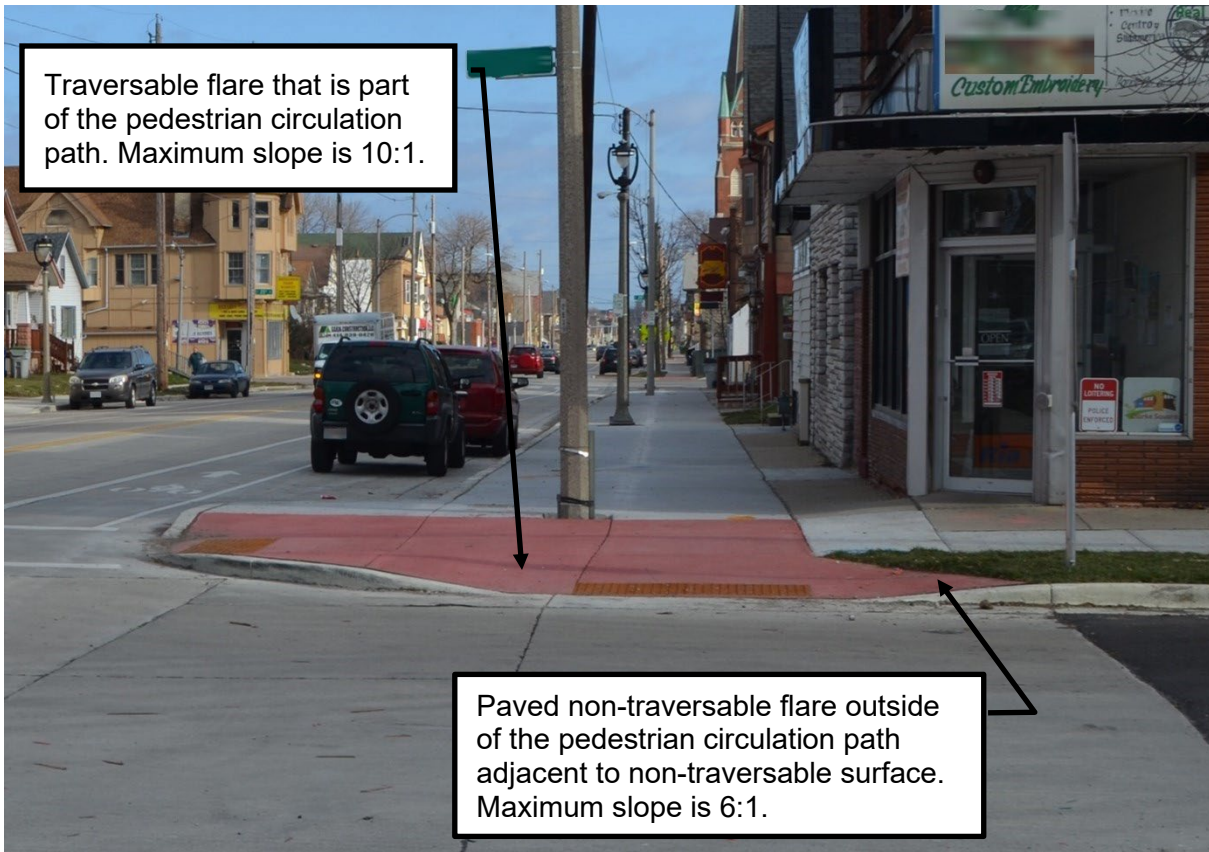
Figure 10.15 Traversable and non-traversable flares
