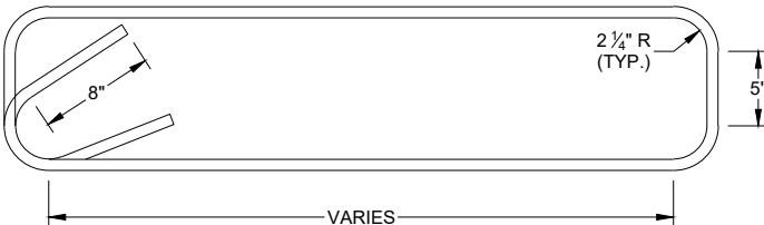
END ANCHOR STIRRUP BAR BENDING DETAIL
