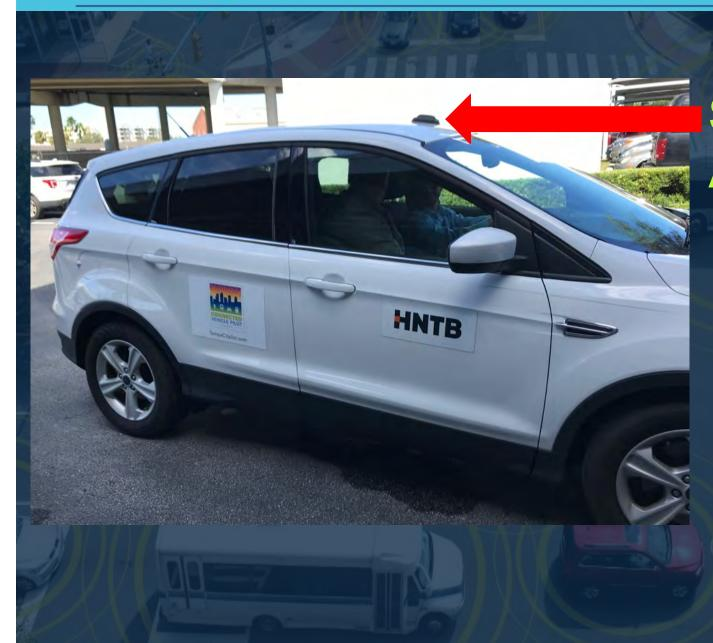
Smart Antenna • SiriusXM • DSRC V2I / I2V
