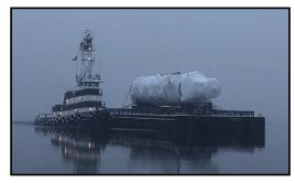
Despite a couple of delays along the way, it took 13 days to transport the mega load, which measured 280 feet long, 16 feet wide and more than 15 feet high, 1,600 miles through six states – Oklahoma, Kansas, Nebraska, South Dakota, Minnesota and Wisconsin – at a maximum speed of 35 mph. When the mega load entered Wisconsin, people, including school children, gathered along the streets to watch as the police-escorted convoy passed.
