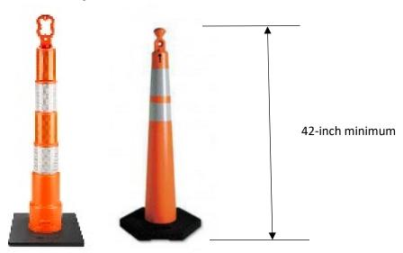
For speeds 40 mph or more, drums shall be spaced 50 feet apart in tapers and 100 feet apart in longitudinal sections. Cones shall not be used in tapers and spaced 50 feet apart in longitudinal sections. For speeds 35 mph or less, drums shall be spaced 25 feet apart in tapers and 50 feet apart in longitudinal sections. Cones shall not be used in tapers and spaced 25 feet apart in longitudinal sections.
