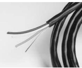
Opticom<sup>™</sup> Model 138 Detector Cable is 0.3 in. (7.62 mm) in diameter and is suitable for direct burial as well as in conduit and exposed overhead installation.\*
