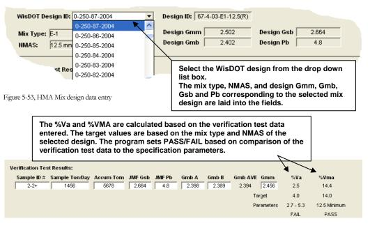
Figure 5-54, Verification test result entry
