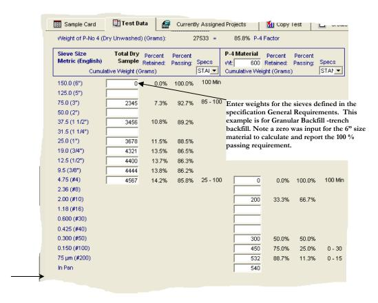
Figure 5-9, Granular Backfill Gradation Worksheet
