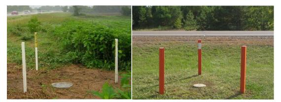
c. Occasionally the protective witness posts are broken by mowing and snowplowing equipment. The posts are replaced by the Geodetic Surveys Unit upon notification.
