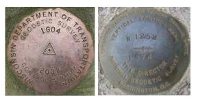
Figure 3. Typical geodetic control disks.
