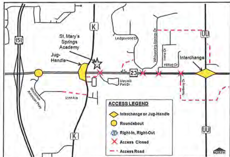
Figure 6 Access Control Between US 151 and County UU
