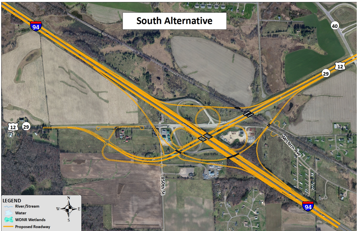
Figure 5: IH 94/US 12/STH 29 Interchange: South Reconstruction Alternative
