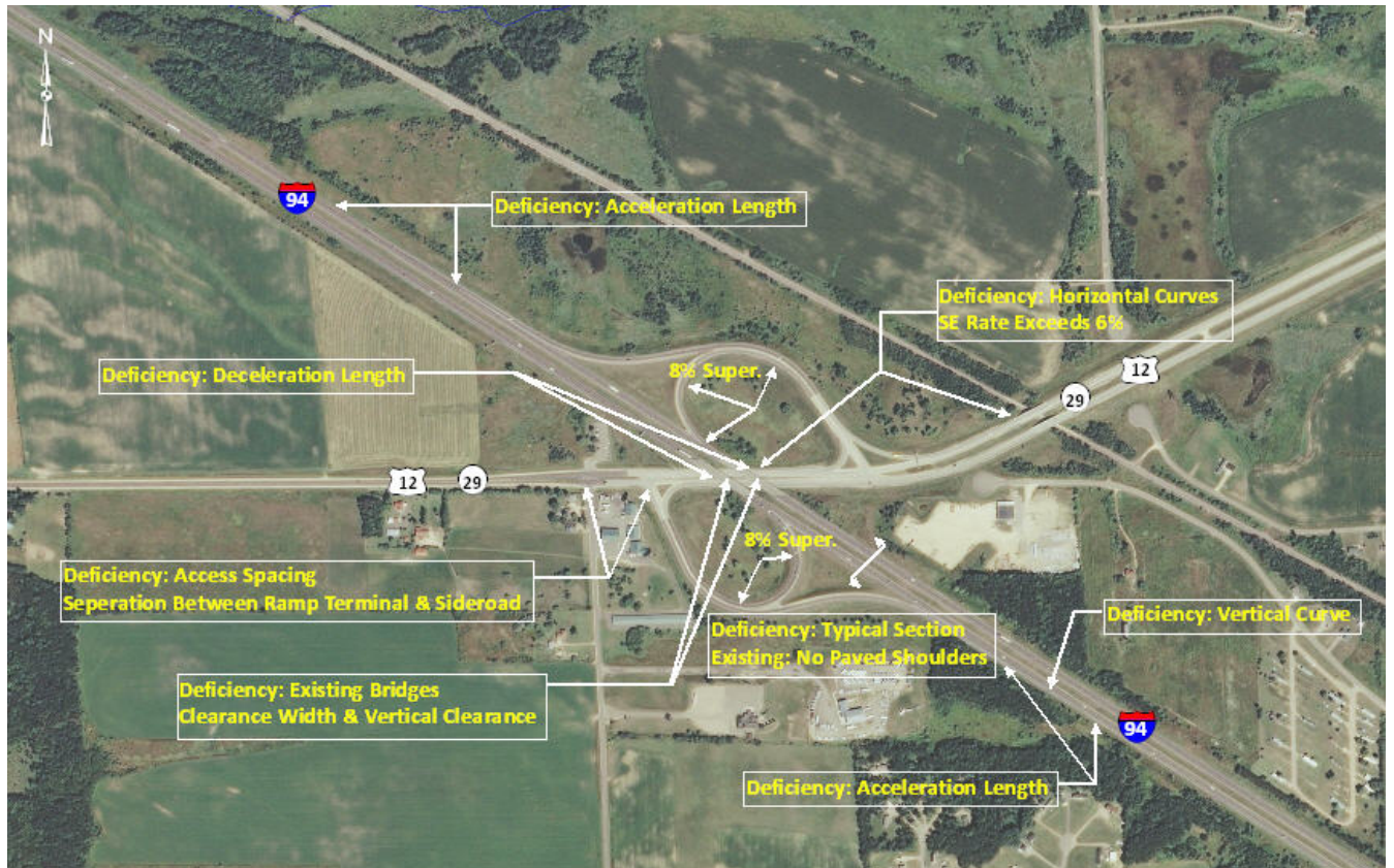
Figure 3: IH 94/US 12/STH 29 Interchange Deficiencies
