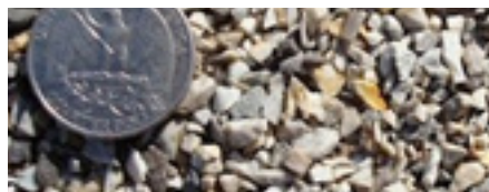
Close-up of typical aggregate used as surface topping in HFST. Source: FHWA
