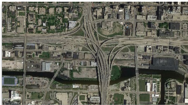
System interchange example (Marquette Interchange)
