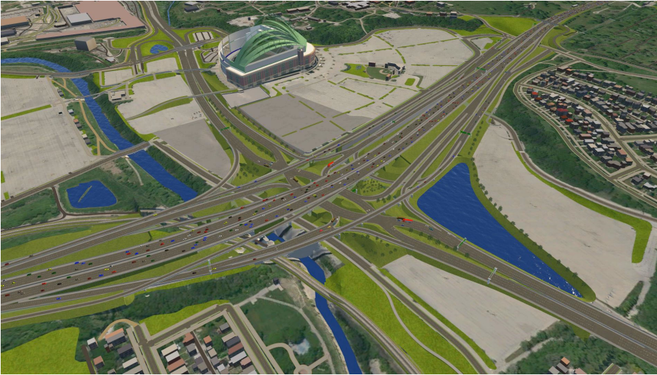
Rendering of the proposed diverging diamond interchange design at the Stadium Interchange.
