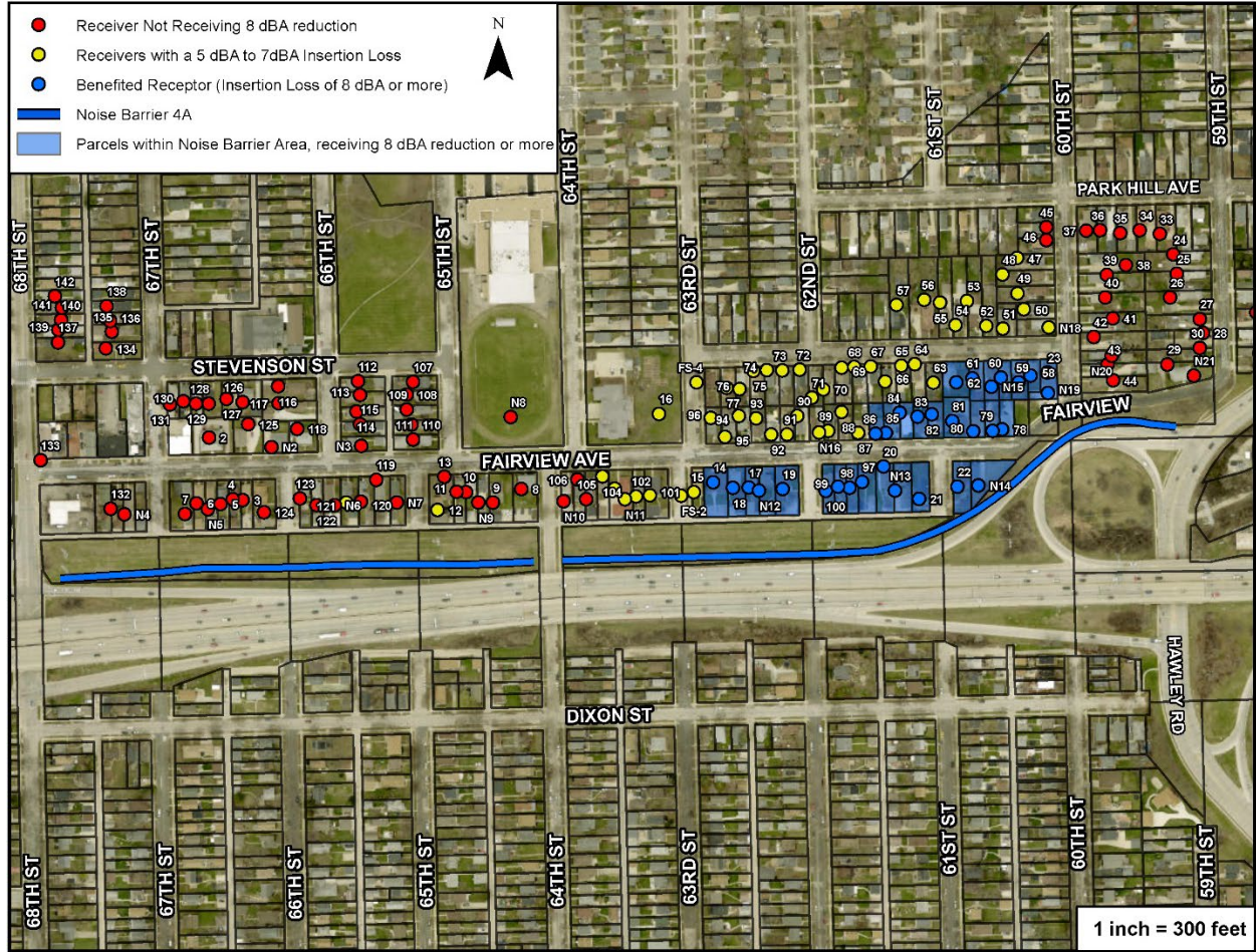
Figure C-5. Barrier 4A Analysis
