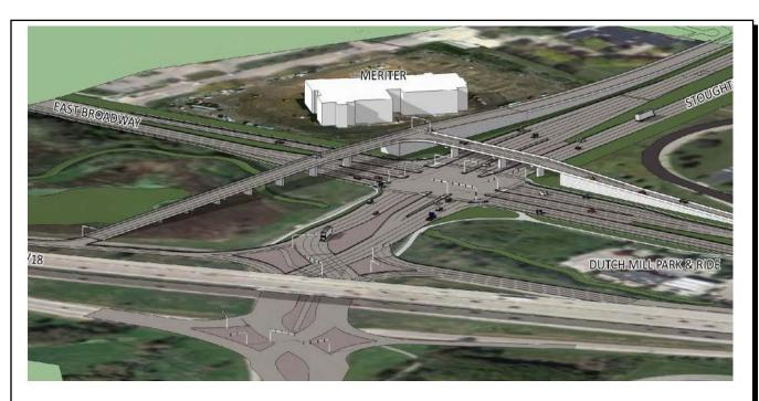
Figure 3.03-1 Grade-Separated Ramp Being Evaluated at Broadway/US 51 Intersection (looking northwest)
