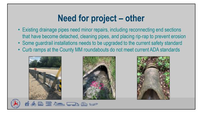
There are other ancillary features of the roadway that require repairs to prevent small issues from becoming more significant. These include drainage pipes, guardrail and curb ramps.
