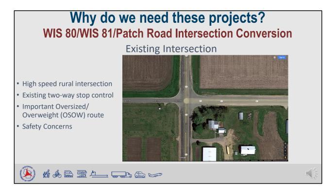
The intersection of Highway 80, Highway 81, and Patch Road is currently a two-way stop control for eastbound and westbound traffic. The intersection is an important oversized overweight route for the State of Wisconsin. As previously discussed, this intersection has a history of severe crashes.
