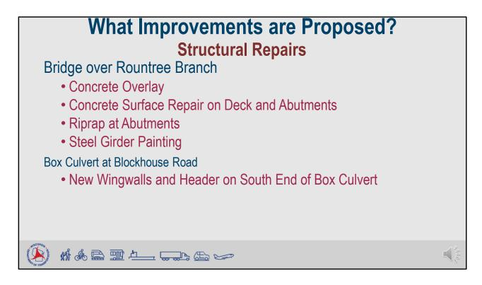
At the bridge over Rountree Branch, the proposed project would install a concrete overlay on the bridge deck to extend the structure's service life. The steel girders would receive spot painting, and the deck underside and abutments would have the damaged concrete spot repaired. The erosion concerns at the abutments would be addressed with the addition of riprap. At the box culvert at Blockhouse Road, the damaged wingwalls and header would be fully replaced.
