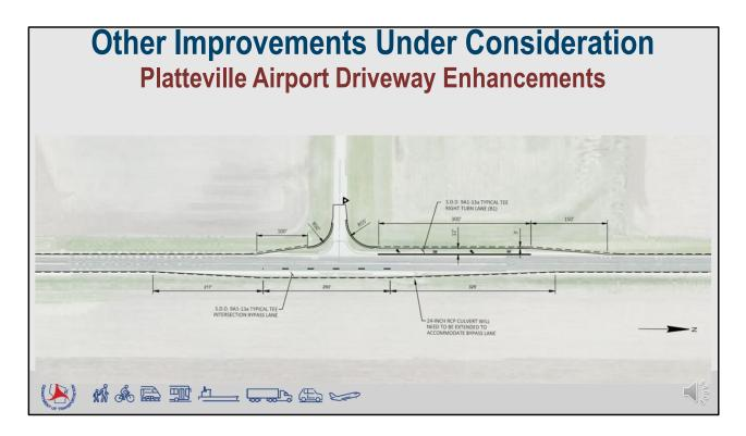
At this time, WisDOT and the City of Platteville are also considering possible driveway enhancements at the Platteville Airport. Potential improvements may include the addition of a left turn bypass lane in the Northbound direction and a right turn lane in the Southbound direction. Improvements for the Platteville Airport driveway would be funded at 100% City cost since there is not a pronounced crash history or roadway deficiency at this location.
