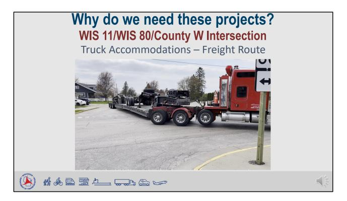
This video shows a DST Lowboy attempting to navigate the existing intersection Eastbound to Northbound. The vehicle does not have room to maneuver through the intersection without significant encroachment into opposing lanes of traffic. Also notice how the rear of the trailer is forced to climb the curb and gutter and ride along the sidewalk to complete the turn. Large loads like this frequently use this intersection but lack the room to complete their maneuvers in the existing configuration.
