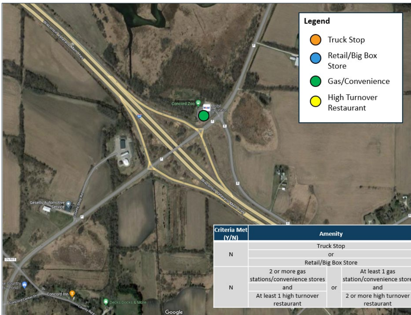
Figure 4-6: Example Exit Not Meeting Wisconsin “Viability” Criteria for Siting NEVI-Compliant EVSE
