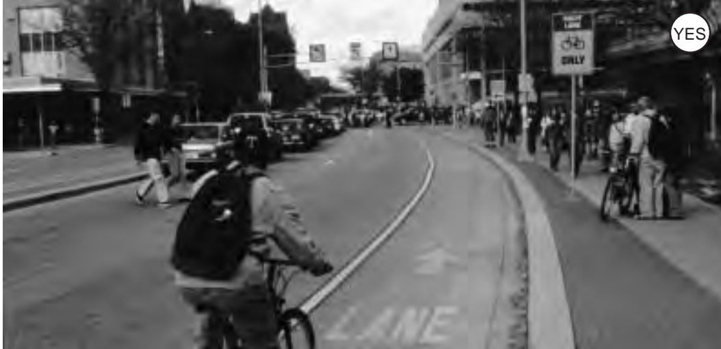
Figure 3-23: The three primary elements that identify a bicycle lane: regulatory signs, lane striping, and pavement markings.
