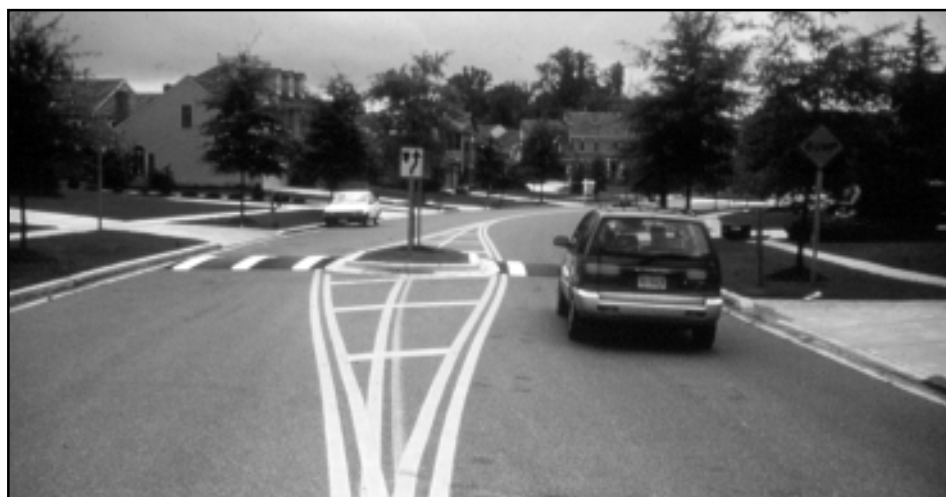
Figure IV.2: Pedestrian medians calm traffic and make crossings safer
