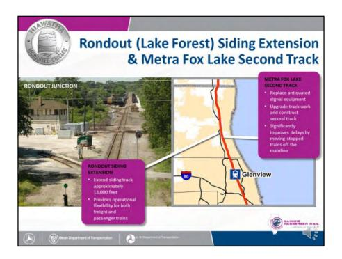
The existing siding on the west side of the mainlines and south of the control point at Rondout in the city of Lake Forest, Illinois is proposed to be extended approximately 13,000 feet to the south to just north of Illinois Route 60. The project would provide operational flexibility for both freight and passenger trains.
