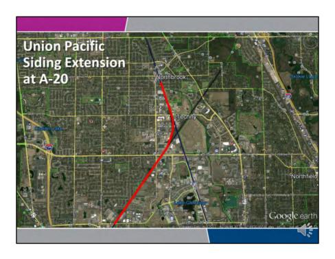
Let's take a closer look at the Union Pacific Siding Extension project. A range of six alternatives was considered to address capacity and delay issues at the Union Pacific junction with the Canadian Pacific at the A-20 control point in Northbrook, IL. Four of the alternatives did not meet the purpose and need of the project and/or had significant environmental impacts associated with them. Two alternatives for the Union Pacific siding projects advanced to the EA.
