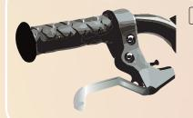
Check your brakes: Make sure that they work. To test this, squeeze on the hand brakes and then try to move your bike forward. If the wheels do not move, they work.
