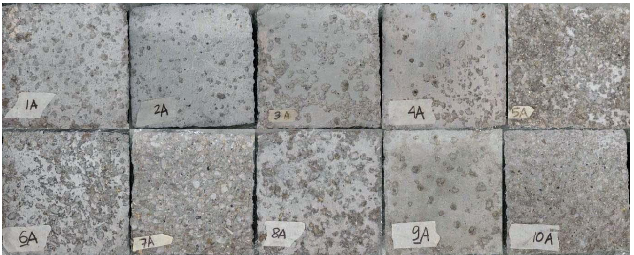
Figure 19. Concrete samples after 30 cycles
