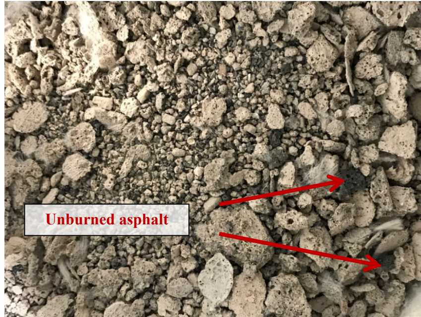
Figure 8 RAS aggregate after ignition at 800°F
