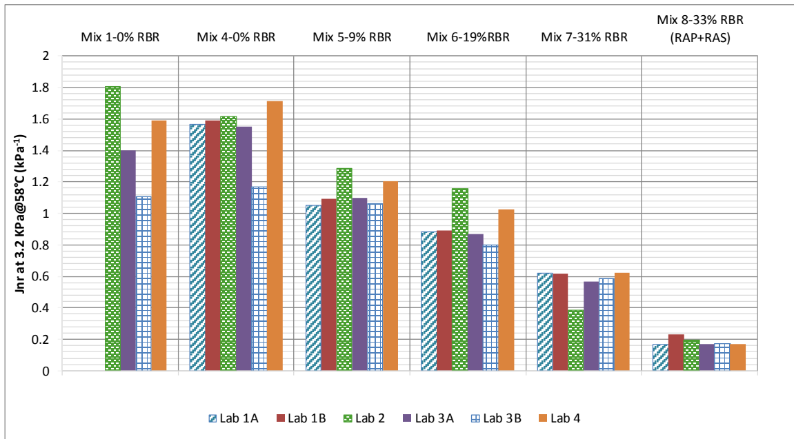
Figure 22 J_{nr} at 3.2 kPa for recovered binders at 58°C
