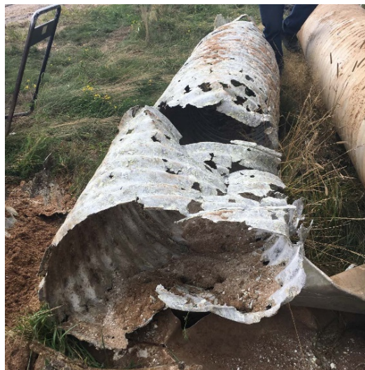
Corroded aluminum pipe removed from WIS 32
