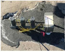
Portable seismic pavement analyzer testing of a repaired pavement section on WIS 66 in Stevens Point "Reliable performance of non-cementitious repair materials will allow for less disruptive, safer, and more cost-effective maintenance of Wisconsin's most heavily traveled highways."
