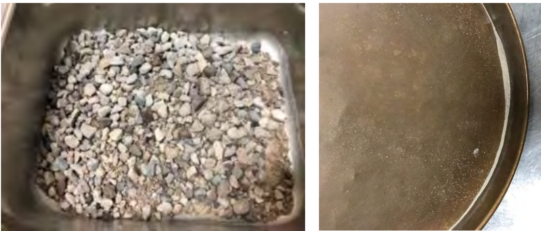
Figure 39: DP Aggregate (Coarse and P200) Material After the Automated Extraction
