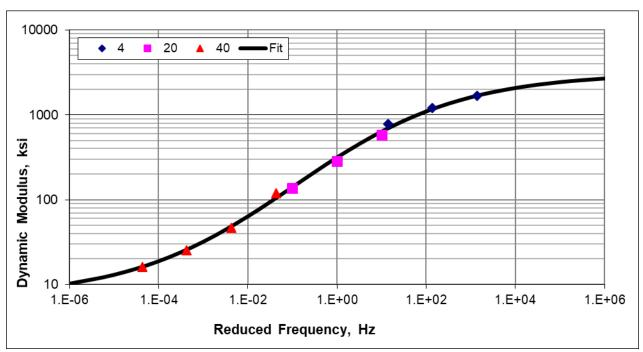
Asphalt Wearing Surface Mixture #0121; PG58-28V, 4 SMA
