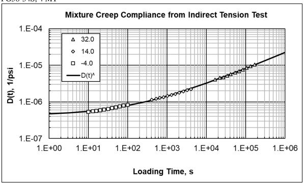
Asphalt Wearing Surface Mixture #0165; IDT Strength – 430 psi. PG58-28S, 4 HT
