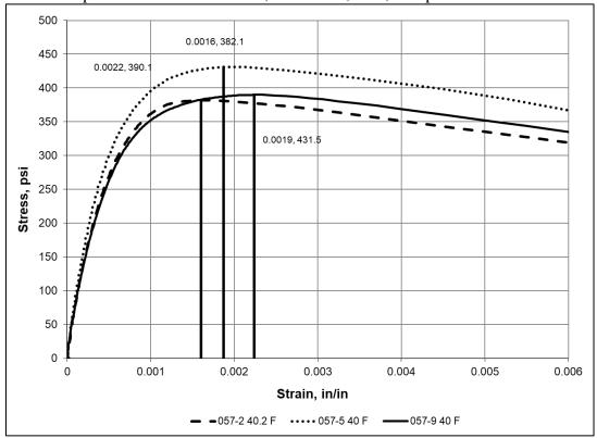
Asphalt Base Mixture #0057; PG58-28S, 3LT; Temperature – 60 °F
