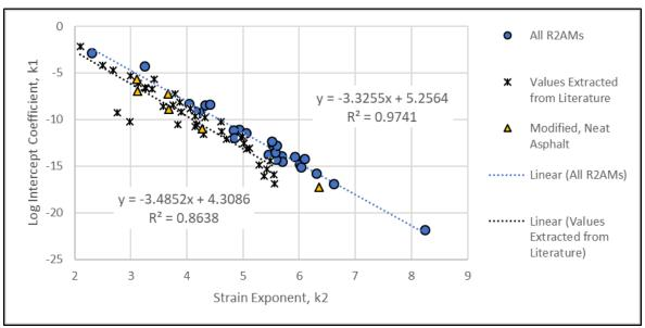
Figure B36. Comparison of the strain exponent and intercept for the R<sup>2</sup>AMs and neat, virgin asphalt mixtures.
