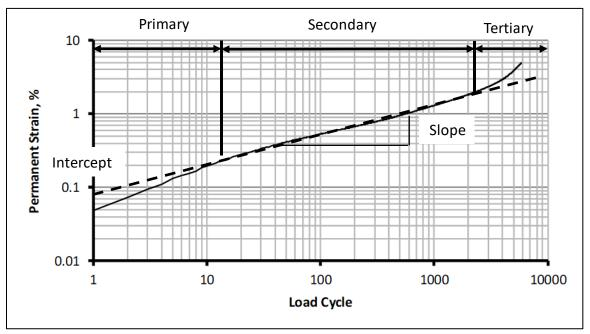
Figure 8. Typical Plastic Strain Curve for an Asphalt Mixtures for a Single Test Temperature in Logarithmic Scale Exhibiting Three Response Zones.
