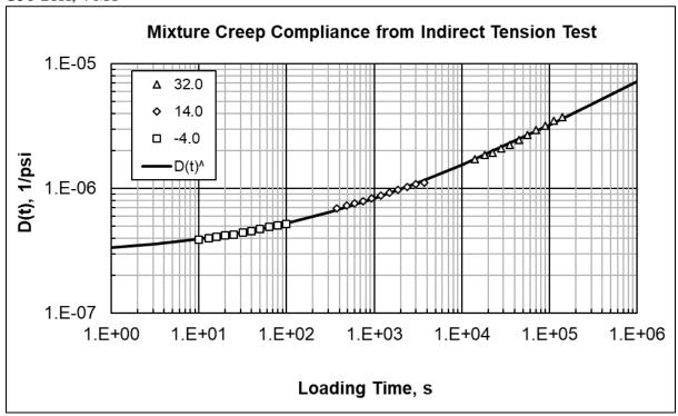
Asphalt Wearing Surface Mixture #1020; IDT Strength – 378 psi. PG58-34V, 4 SMA
