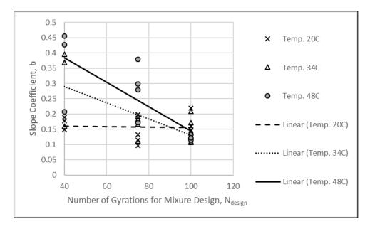
Figure 10. Impact of N<sub>Design</sub> on the Slope Coefficient from the Repeated Load Plastic Strain Test Data.
