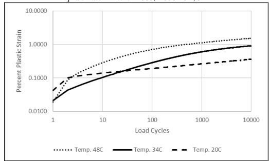
Asphalt Wearing Surface Mixture #0121; PG58-28V, 4 SMA
