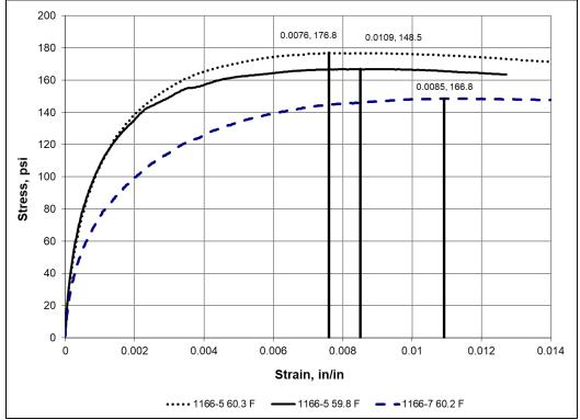
Asphalt Base Mixture #1166; PG58-28S, 2 HT; Temperature – 80 °F
