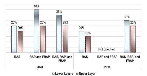
Figure 1. Maximum Allowable Percent Binder Replacement Specified in the 2020 and 2010 WisDOT Standard Specifications.
