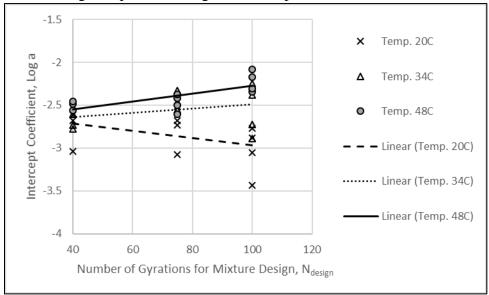
Figure 9. Impact of N<sub>Design</sub> on the Intercept Coefficient from the Repeated Load Plastic Strain Test Data.
