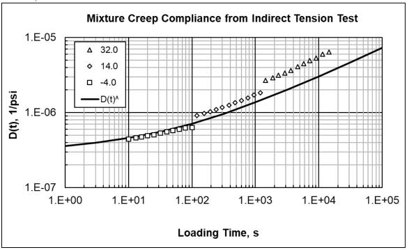
Asphalt Wearing Surface Mixture #8357; IDT Strength - 398 psi. PG58-34S, 4 LT
