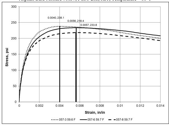
Asphalt Base Mixture #0057; PG58-28S, 3LT; Temperature – 80 °F
