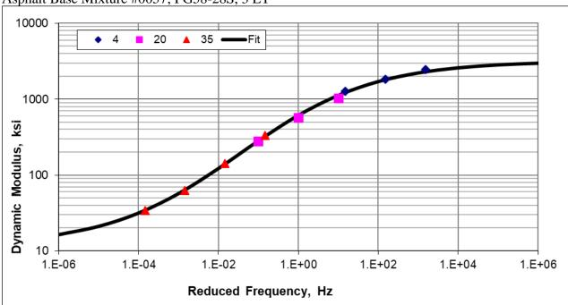
Asphalt Base Mixture #0119; PG58-28S, 3 HT
