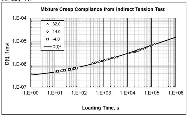
Asphalt Wearing Surface Mixture #0319; IDT Strength -465~psi. PG58-28H, 4 MT
