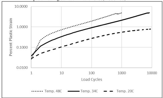
Asphalt Wearing Surface Mixture #0236; PG58-28S, 4 MT
