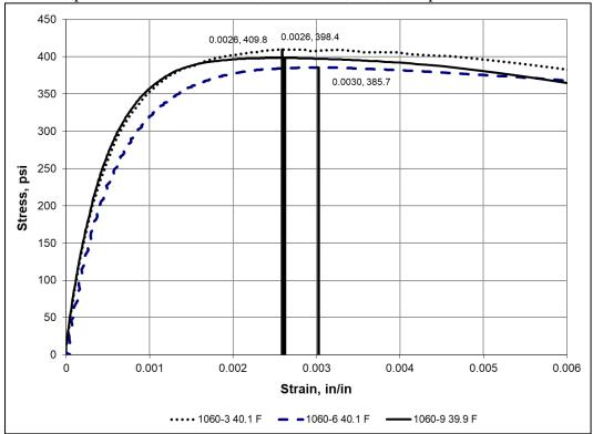
Asphalt Base Mixture #1060; PG58-28H, 3HT; Temperature – 60 °F
