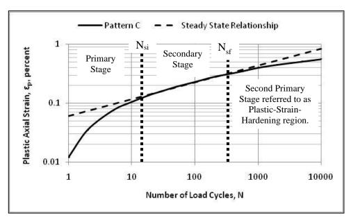
Figure G39. Pattern C typical plastic strain curve for an asphalt mixture in logarithmic scale.
