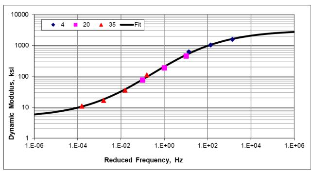
Asphalt Wearing Surface Mixture #0236; PG58-28S, 4 MT
