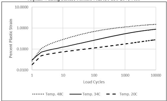
Asphalt Wearing Surface Mixture #0258; PG58-28S, 4 MT
