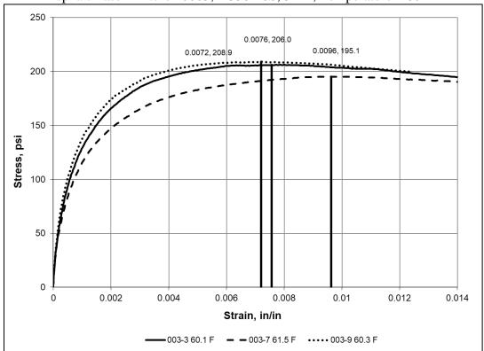
Asphalt Base Mixture #0003; PG58-28S, 3MT; Temperature – 80 °F:
