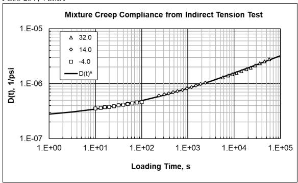
Asphalt Wearing Surface Mixture #0127; IDT Strength – 417 psi. PG58-34S, 4 MT
