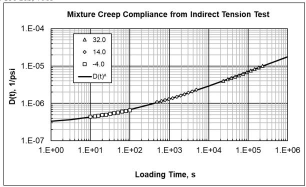
Asphalt Wearing Surface Mixture #0258; IDT Strength – 457 psi. PG58-28S, 4 MT
