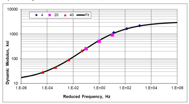
Asphalt Wearing Surface Mixture #0165; PG58-28S, 4 HT
