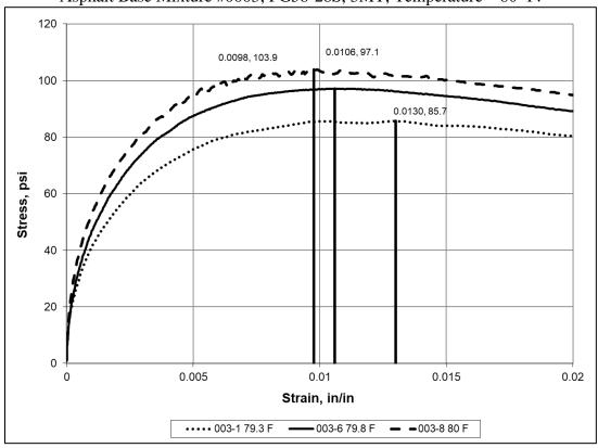
Asphalt Base Mixture #0057; PG58-28S, 3LT; Temperature – 40 °F
