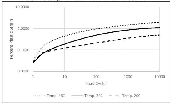
Asphalt Wearing Surface Mixture #0208; PG58-28S, 4 LT
