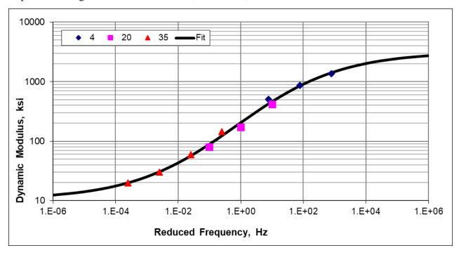
Asphalt Wearing Surface Mixture #0319; PG58-28H, 4 MT
