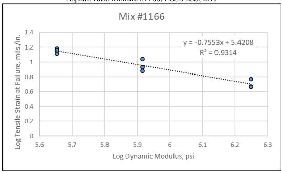
Asphalt Base Mixture #1166; PG58-28S, 2HT
