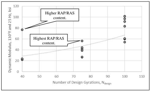
Figure 2. Graphical Comparison of  $N_{design}$  Gyrations and Dynamic Modulus Measured at  $130^{\circ}F$  (54.4  $^{\circ}C$ ) and 25 Hz.
