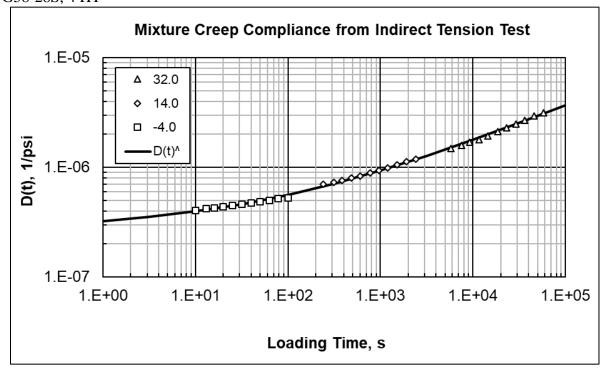
Asphalt Wearing Surface Mixture #0208; IDT Strength – 358 psi. PG58-28S, 4 LT
