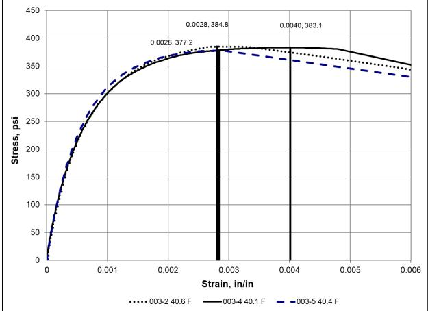
Asphalt Base Mixture #0003; PG58-28S, 3MT; Temperature – 60 °F:
