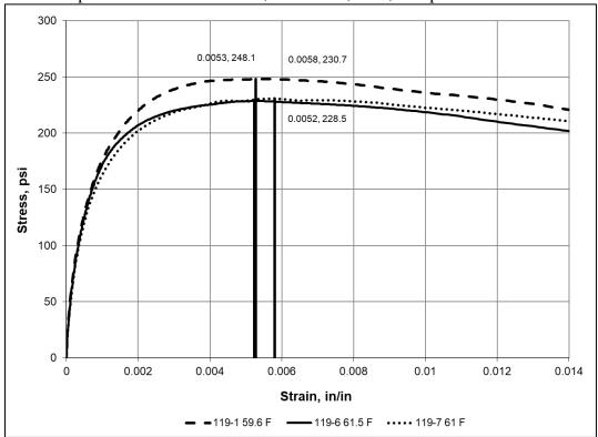
Asphalt Base Mixture #0119; PG58-28S, 3HT; Temperature – 80 °F
