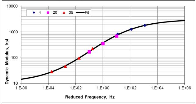
Asphalt Wearing Surface Mixture #0093; PG58-28H, 4 HT
