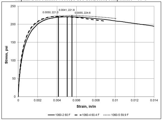
Asphalt Base Mixture #1060; PG58-28H, 3HT; Temperature – 80 °F
