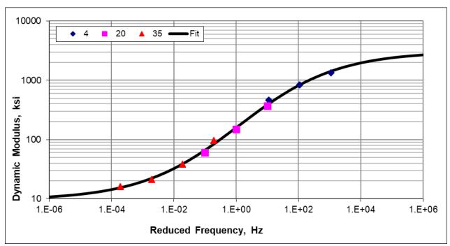
Asphalt Wearing Surface Mixture #7130; PG58-34V, 5 HT
