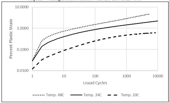
Asphalt Wearing Surface Mixture #0251; PG58-28V, 4 HT
