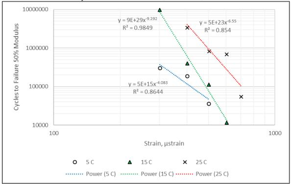
Asphalt Base Mixture #1166; PG58-28S, 2HT
