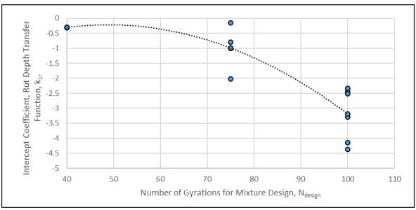
Figure 14. Correspondence between  $N_{Design}$  and the Intercept Coefficient,  $k_{Ir}$ .
