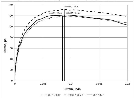
Asphalt Base Mixture #0119; PG58-28S, 3HT; Temperature – 40 °F
