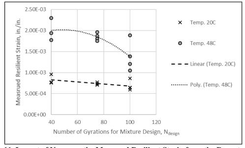
Figure 11. Impact of N<sub>Design</sub> on the Measured Resilient Strain from the Repeated Load Plastic Strain Test Data.
