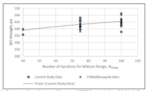
Figure 13. Correspondence between N<sub>Design</sub> and IDT Strength from Multiple Data Sources.
