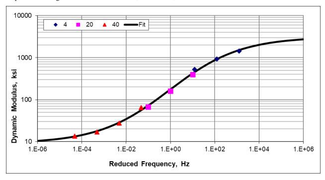
Asphalt Wearing Surface Mixture #0251; PG58-28V, 4 HT
