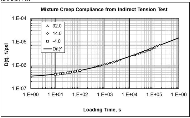
Asphalt Wearing Surface Mixture #0236; IDT Strength – 481 psi. PG58-28S, 4 MT
