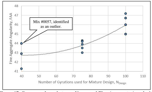
Figure 17. Correspondence between N<sub>Design</sub> and Fine Aggregate Angularity
