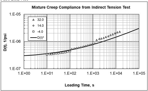
Asphalt Wearing Surface Mixture #0121; IDT Strength – 448 psi. PG58-28V, 4 SMA
