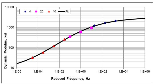
Asphalt Wearing Surface Mixture #0258; PG58-28S, 4 MT
