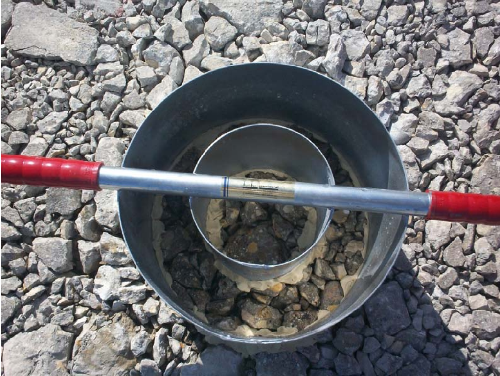
Figure 21. Result of permeability test trial
