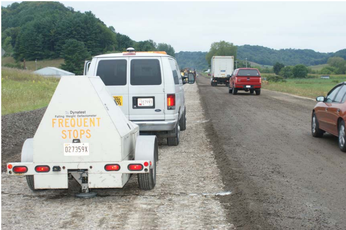
Figure 18. FWD testing of a joint
