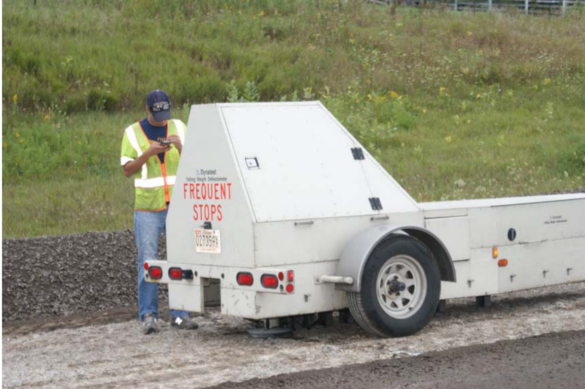
Figure 17. Gathering GPS location of joint during FWD testing
