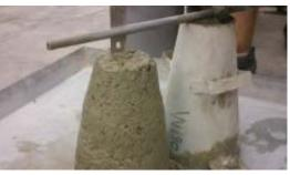
Testing the workability of concrete mixture using a slump cone
