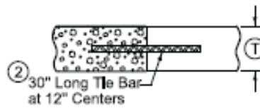
Figure 4-17 Iowa Approach DW Joint (IADOT)
