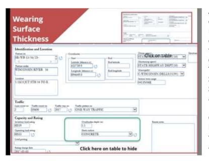
Another common error involves the overlay thickness. Inspectors are responsible with accurately reporting the depth of any overlays on the inspection form, and are encouraged to verify the overlay thickness during each inspection. The results are entered into the Highway Structures Information System on the Structure Information Tab, along with the appropriate deck surface material.
