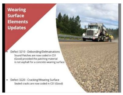
There are a couple of changes to the Wisconsin Structure Inspection Field Manual in the last few years regarding wearing surface defects. First, wearing surfaces that have been patched where the patches are sound are to be coded in CS1 or Good condition for that area. The only exception to that is when asphalt patching materials have been used on a concrete wearing surface. Those patches are considered unsound and Should be coded in CS3 or Poor condition.
