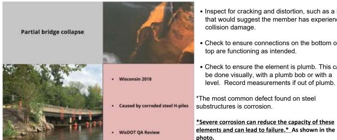
You're now seeing images from the partial collapse of a local 3 span bridge in Wisconsin that occurred in 2018. The steel H-piles at the piers had severe corrosion and buckled under load. Because of this partial bridge collapse WISDOT conducted Quality assurance reviews on a subset of bridges composed of steel piles and columns statewide. From the review, several piles were found to be in severe condition that would be considered condition state 4.
