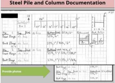
When section loss appears to be greater than 5 percent take measurements to determine the actual amount of section loss. When section loss is measured to be greater than 15 percent per element a sketch is required. This sketch should include percent section loss at each location on the element including the size and location of voids.
