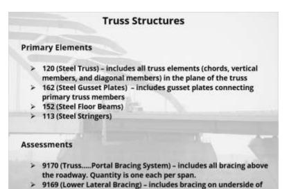
Inspection of truss superstructures are documented using four primary elements and two assessments to account for all the structural steel.
