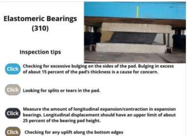
Expansion elastomeric bearings made of neoprene rubber and generally are thick rectangular pads that accommodate longitudinal and rotational superstructure movements.
