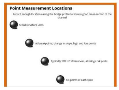
There must be enough point locations along the bridge profile to show a good crosssection of the channel. The point measurements along the bridge profile must capture the high and low points at reasonable intervals. The point measurements must be taken at the substructure units, at breakpoints (changes in slope/high & low points) between the substructure units, and at spacing typically of 10' to 15' intervals or ¼ points of each span or at the bridge rail posts.
