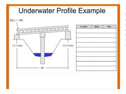
The intent of the underwater profile is to have a repeatable procedure for future comparisons. It is not necessary for the inspector to determine the true elevation of the stream bed or water elevation so long as the same methods are repeated from the same locations at every inspection.
