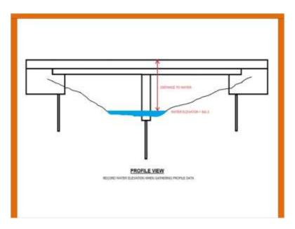
Reference the water surface elevation to a known elevation on or near the bridge.
