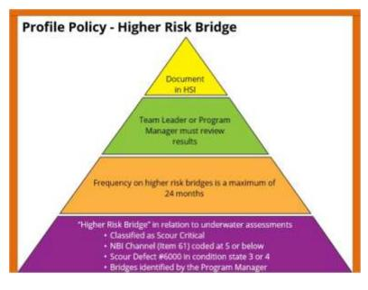
The underwater profile must continue on bridges considered as "higher risk". Higher risk bridges are defined as those classified as Scour Critical - these are bridges determine by evaluation or observation to be vulnerable to scour; those with an NBI Channel (Item 61) coded at 5 or below; those with a Scour Defect #6000 in condition state 3 or 4; and those identified by the program manager.
