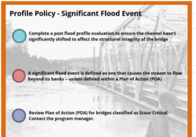
Structures over water that experience a significant flooding event must have a post flood profile evaluation to ensure the channel hasn't significantly shifted to affect the structural integrity of the bridge.
