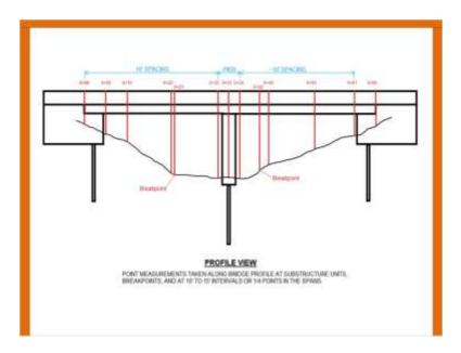
This drawing shows example locations of point measurements along the bridge profile: at substructure units, at breakpoints, at spacing of 10' along the bridge.
