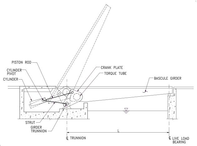
Figure 3.2.6-1: Bascule Without Counterweight – Hydraulic Cylinder Drive.
