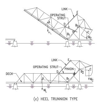
Figure 3.2.4-1: Types of Strauss Bascule Bridges.
