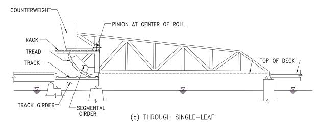
Figure 3.2.3-1: Types of Scherzer Rolling Lift Bascules.
