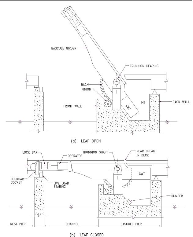
Figure 3.2.2-1: Single Leaf Simple Trunnion Bascule.
