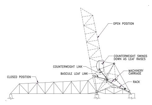
Figure 3.2.5-1: Through-Truss ABT Bascule.
